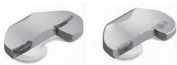
Fig. 1: Subsurface stresses for two different degrees of congruency
