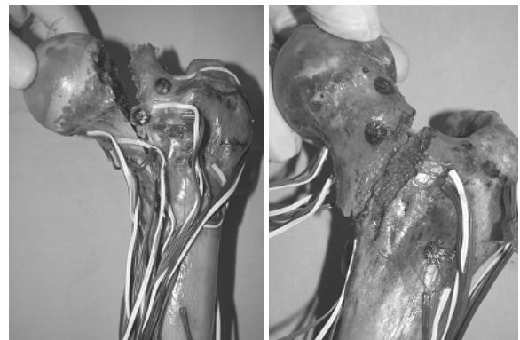
Fig. 2 – Failed intact femurs, showing a variety of fractures ranging from sub-capital (left) and neck base (right).
