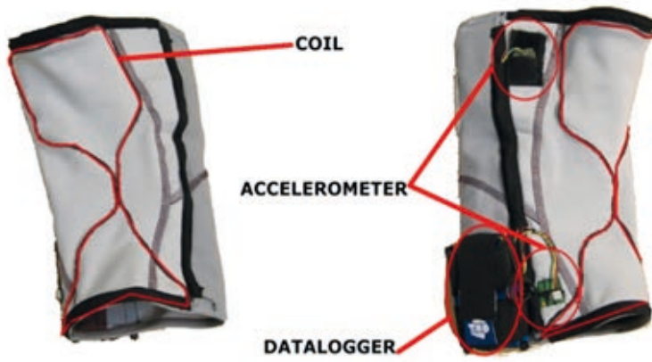
Smart Knee Brace showing the hardware configuration.
