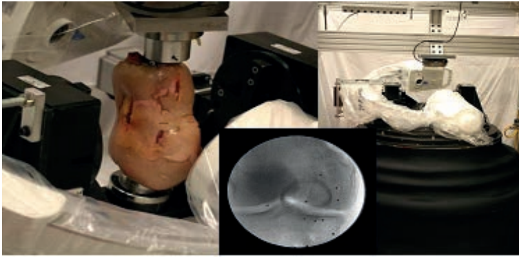
Robotic knee manipulator, and C-arm, used to track implant motion during simulated activities
