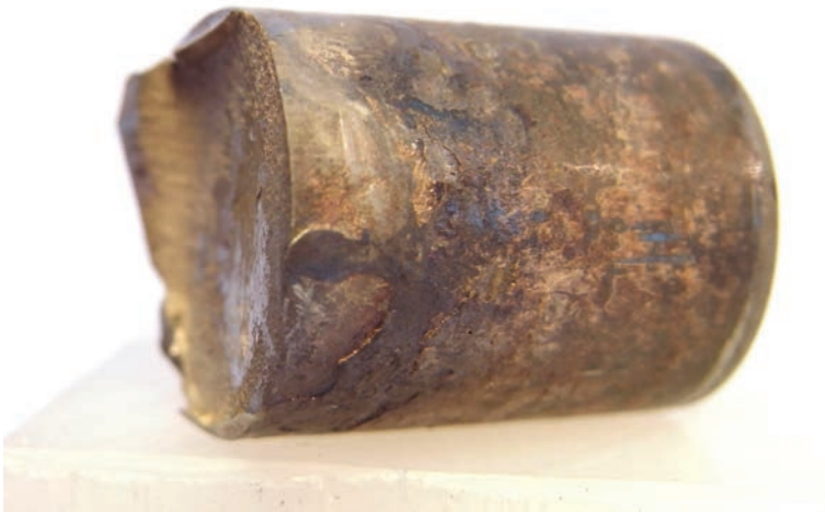
-A fractured modular Titanium/Titanium junction
