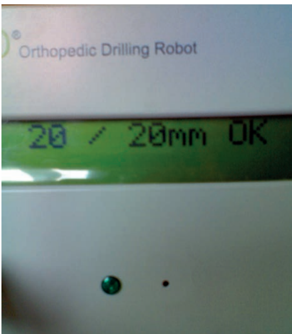
Fig.3. Real time information on the display. The right number (20 mm) is preliminary set
